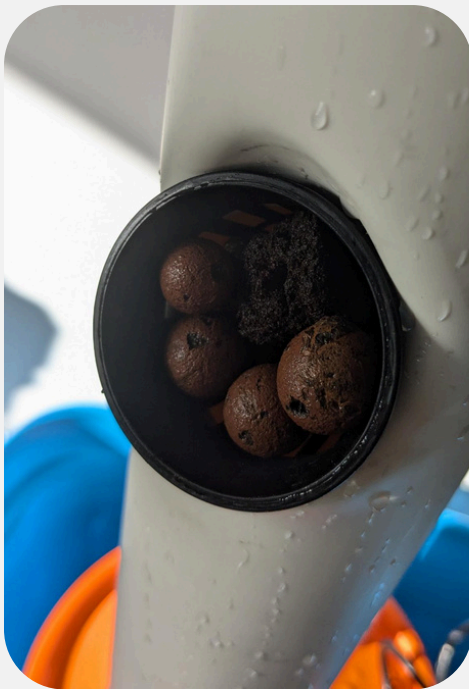
Figure 1. Kits were designed and constructed by the UFV research team. They included an aquarium pump, two PVC towers with hand-cut pockets, tubing, and nutrients, with a total of 14-16 grow cups. The test kit was trialed at two of the researcher team's homes.
